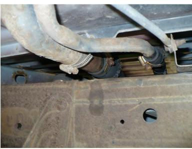
Next remove the two hose clamps holding the filler tube and vent tube and loosen the two hoses a little so they will come off easier later.
