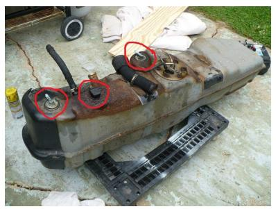
This is the tank removed. Notice the three sensors on the top. (two grey and one black)
