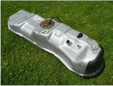
This is the new tank with all of the sensors, plastic end cover and fuel pump assembly installed. I did not get a picture with the plastic strap tape on the tank.
