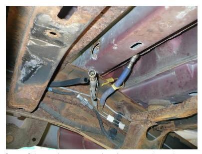
Here are the fuel lines and one of the sensor hoses disconnected. I kept the fuel line upright so no gas would come out of them. To disconnect the fuel lines you either need a tool that you can get at just about any auto parts store or if you have to you can make a tool out of just about anything that is stiff and will wrap around the hose that you can push into the connector. I had a tool but it was the wrong size so I made one out of a piece of a plastic wire clamp like this.
