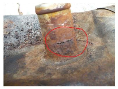
This is where the crack was in my tank. It was just at the end of where the filler tube hose ended.
