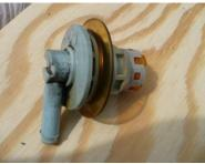
These are the sensors removed from the tank. There are two of the grey ones and one black one. Make sure you put them back in the same spot on the tank.
