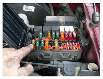
Then remove the fuse for the fuel pump in the fuse box under the hood in the engine compartment. It is the 20amp fuse where I am pointing to in the picture. Check you manual for a better description on fuse locations.
